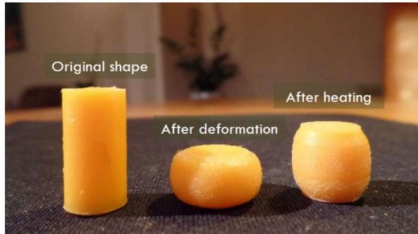
Figure 55: Below the glass temperature a polymer can be deformed but will not forget its original shape.
