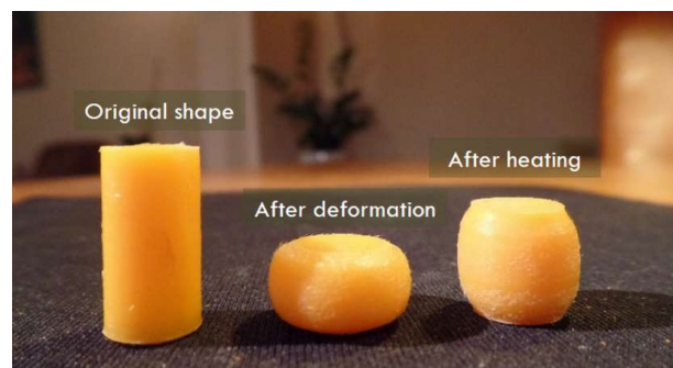
Figure 17: Below the glass temperature a polymer can be deformed but will not forget its original shape.
