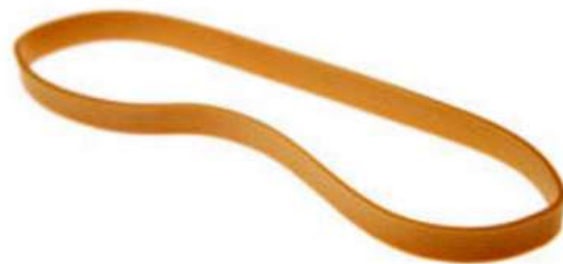
Figure 26: Elastic band made from a polymer in the rubber phase.
