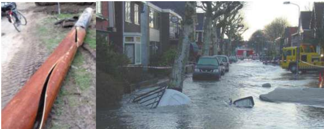
Figure 61: Aging can cause a polymer pipe for water supply to suddenly break.
