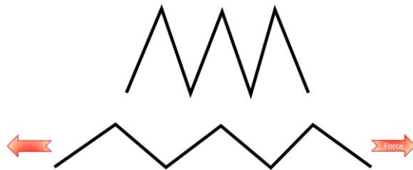
Figure 16: Rotation of chain segments results in a large deformation. The relative position of the molecules does not change.
